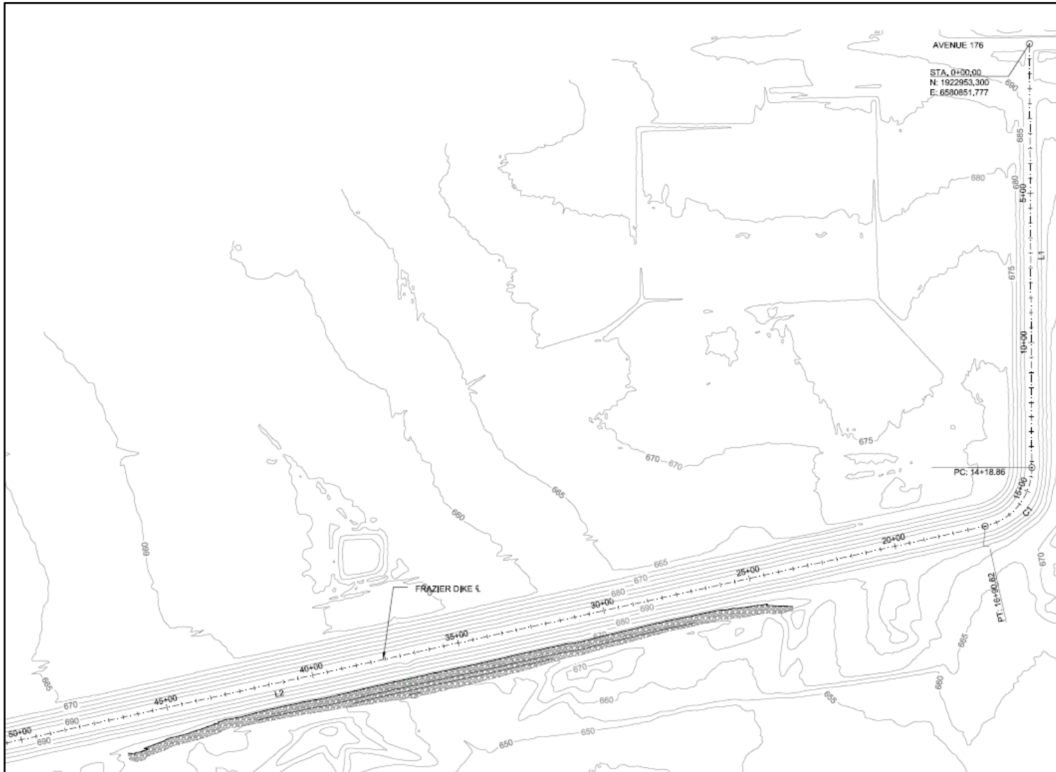
Figure 8. Design of rock revetment placement along Frazier Dike, shown as dark grey hashed section.
